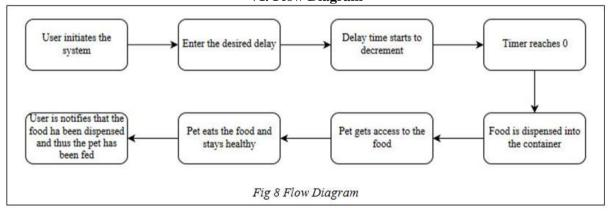
System will be powered up by the user. Desired delay time will be entered by the user, after which dispensing will take place. Now the delay time will start decrementing and will finally reach termination. When the delay timer reaches 0, food will be dispensed into the container. Pet gets access to the food. User is notified and thus is satisfied that the pet has been fed.
